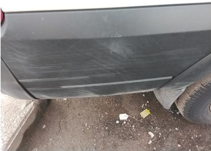
43: Qtr Panel Moulding os Scuffed (Unpainted) Over 100mm
