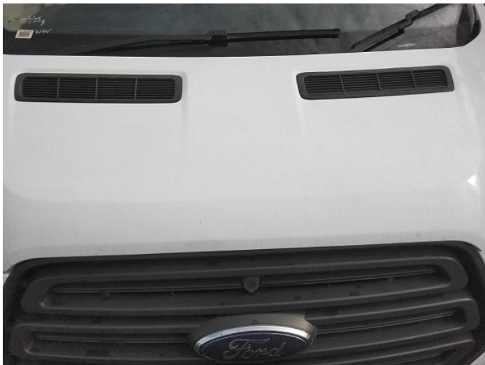
1: Bonnet Chipped Multiple Chips
