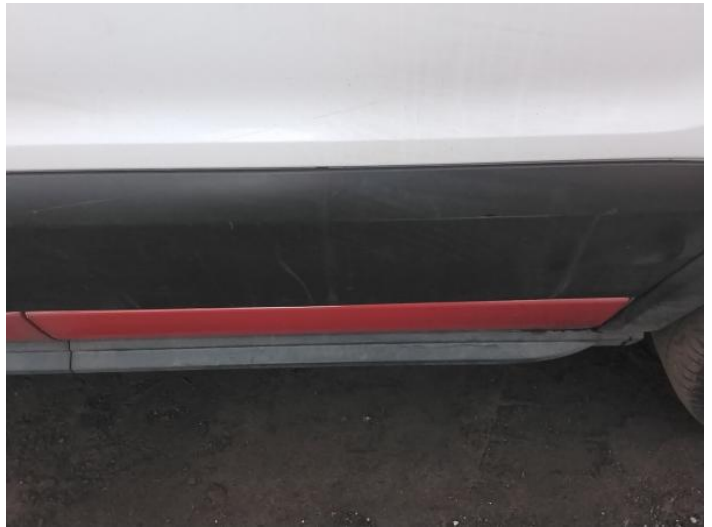
54: Door Moulding osf Scuffed (Unpainted) Over 100mm
