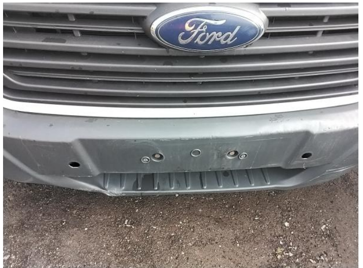
2: Number Plate Front Missing Replace
