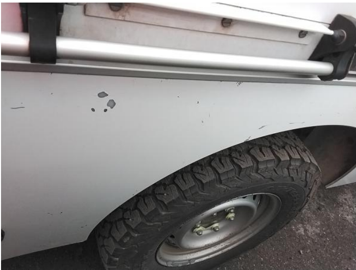
5: Qtr Panel osr Chipped Multiple Chips
