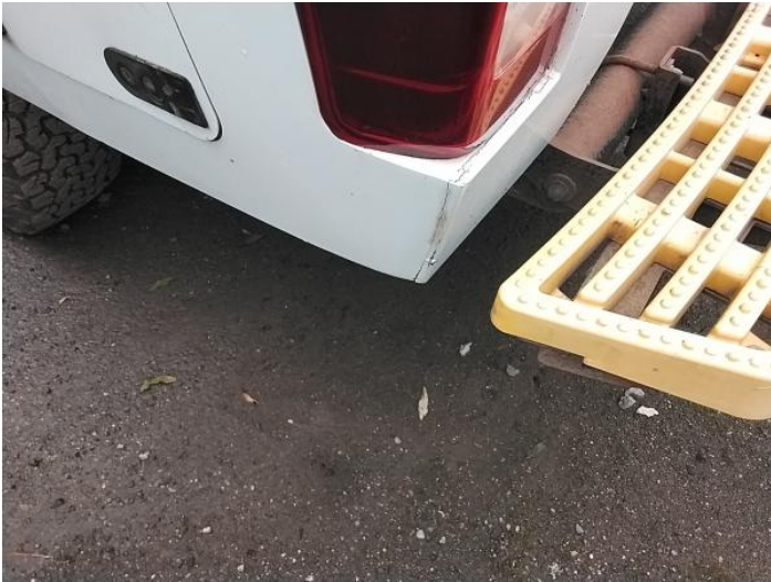
3: Qtr Panel nsr Cracked Replace
