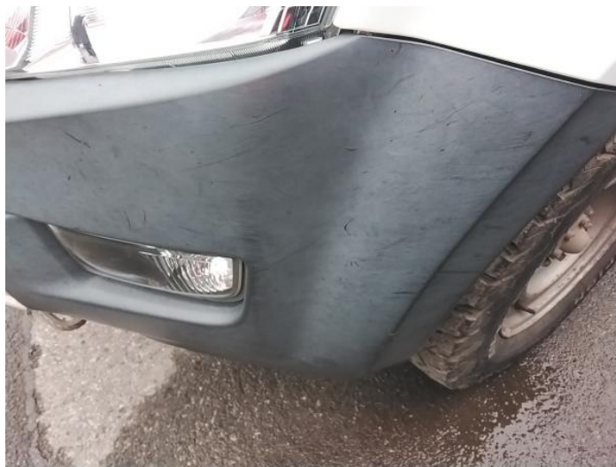
2: Bumper Front Scratched Over 100mm Thru Paint
