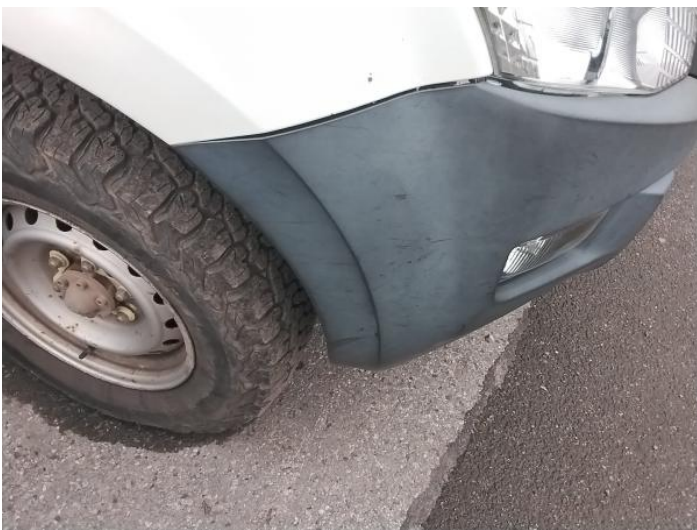
7: Bumper Front Scratched Over 100mm Thru Paint
