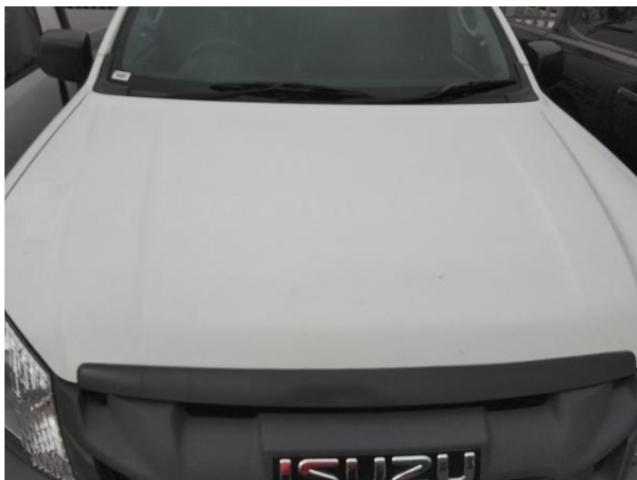
1: Bonnet Chipped Multiple Chips
