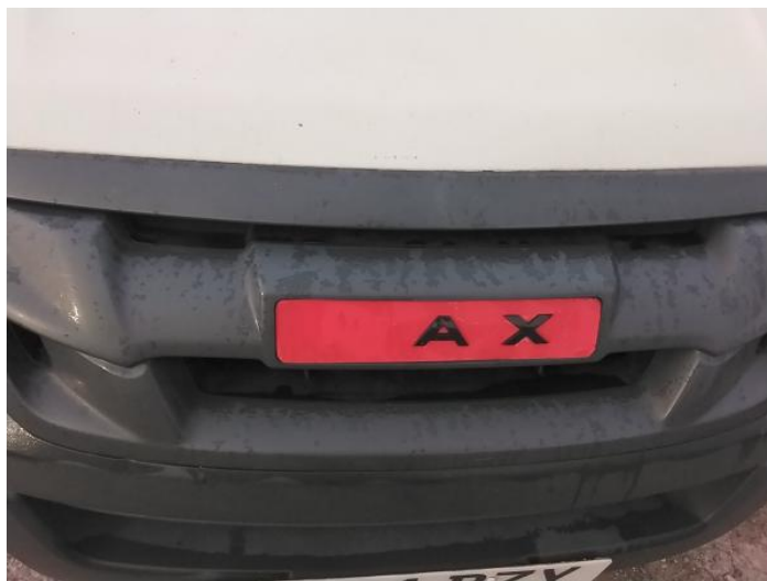
2: Badgedecal Front Missing Replace
