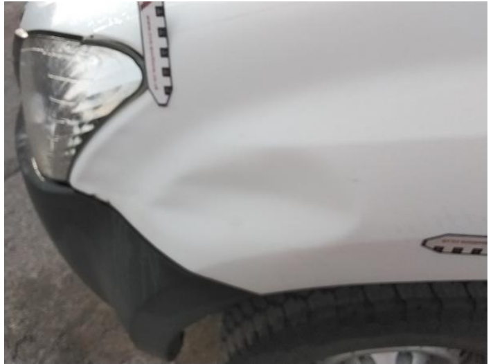
4: Wing nsf Dented Over 30mm
