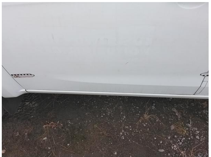
8: Door nsf Scratched Over 25mm Thru Paint
