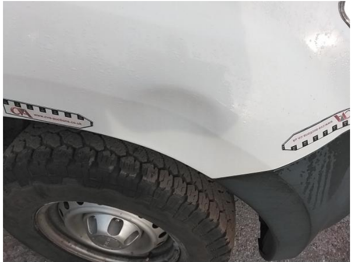
16: Wing osf Dented Over 30mm
