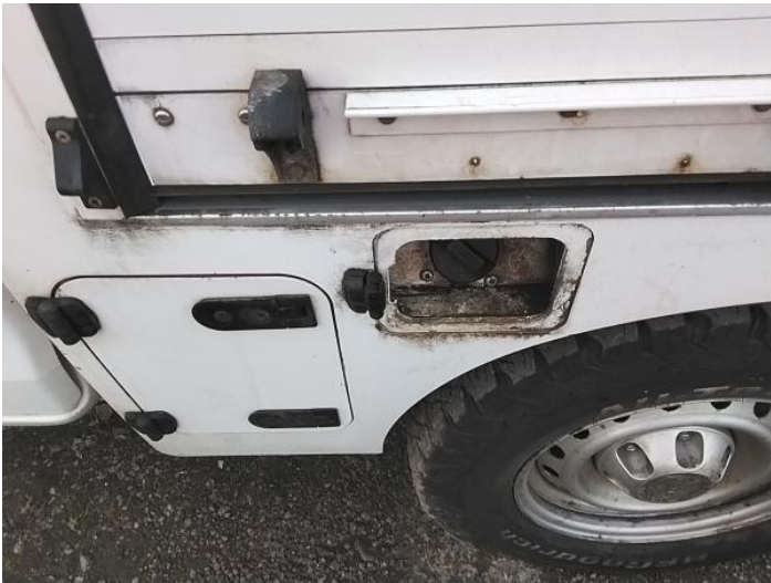
17: Fuel Flap Missing Replace
