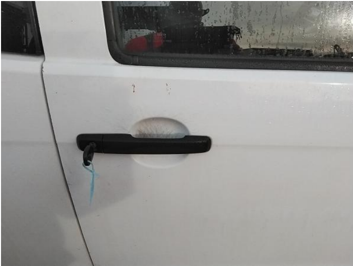
15: Door osf Chipped Multiple Chips
