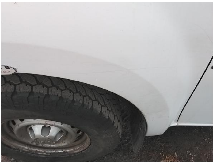
5: Wing nsf Scratched Over 25mm Thru Paint
