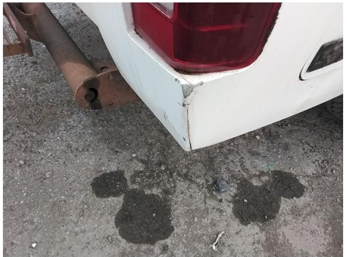
12: Qtr Panel osr Cracked Replace
