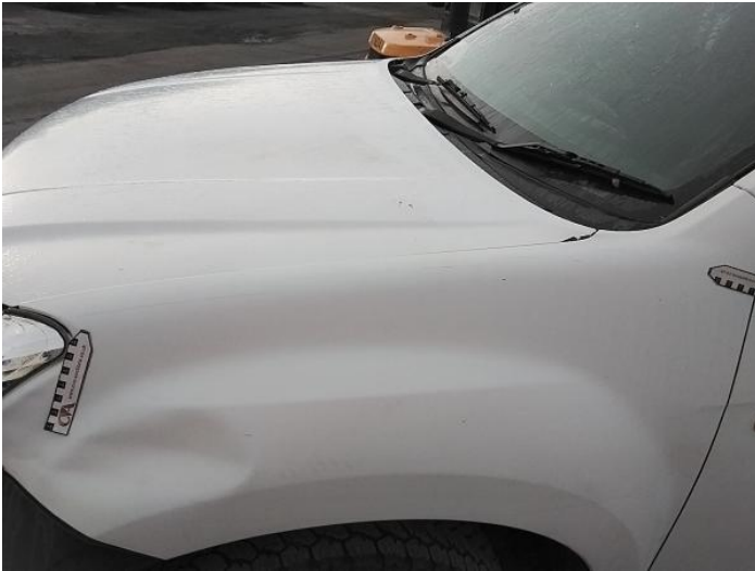
3: Wing nsf Scratched Over 25mm Thru Paint
